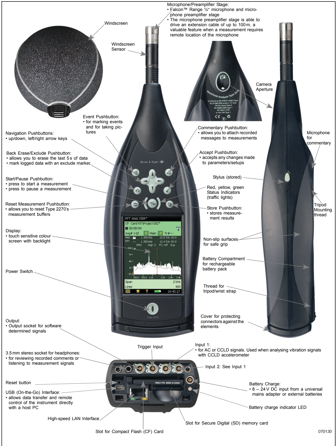
Fig. 4 Key features of Hand-held Analyzer Type 2270
